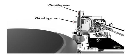
With needle in the record groove, carefully move tonearm up or down with main VTA adjustment crew. When you are satisfied with VTA setting, carefully retighten VTA locking screw and move tonearm to the tonearm rest position.
