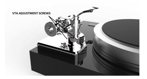
F-Note tonearm has two stage VTA adjustment. Once you set VTA by moving main tonearm pillar up and down, you can unlock fine adjustment with locking screw shown on following illustration.
