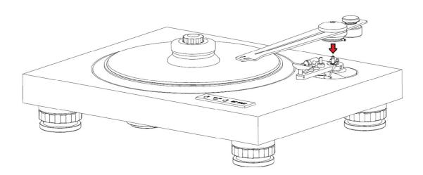
Screw the tonearm connector on the top of the tonearm. Take care about correct position of connector's pins.
