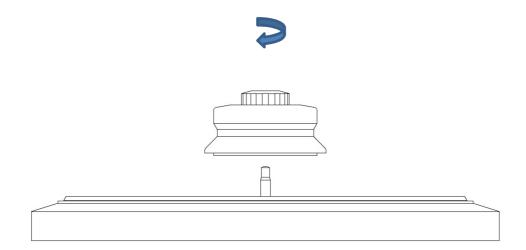
Once you have screwed the record clamp onto the platter, double-check to make sure that the clamp is holding the platter securely. Then grasp the record clamp and use it to carefully lower and center the platter on the sub-platter.
